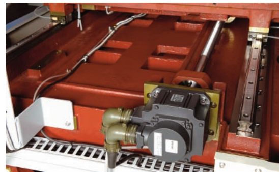
Direct drive and generously dimensioned spindles. The digital AC direct drive system, gives a shaft resolution of 0.05 \mu\text{m} . The spindle is also arranged exactly in the centre of the load in order to ensure "soft" axis movement.
