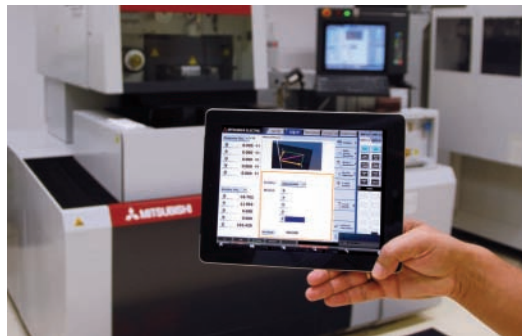
Telecontrol: Remote control via PC. Telecontrol realises the remote monitoring and remote control of the machine from any site. The optimisation of running processes is also possible.
