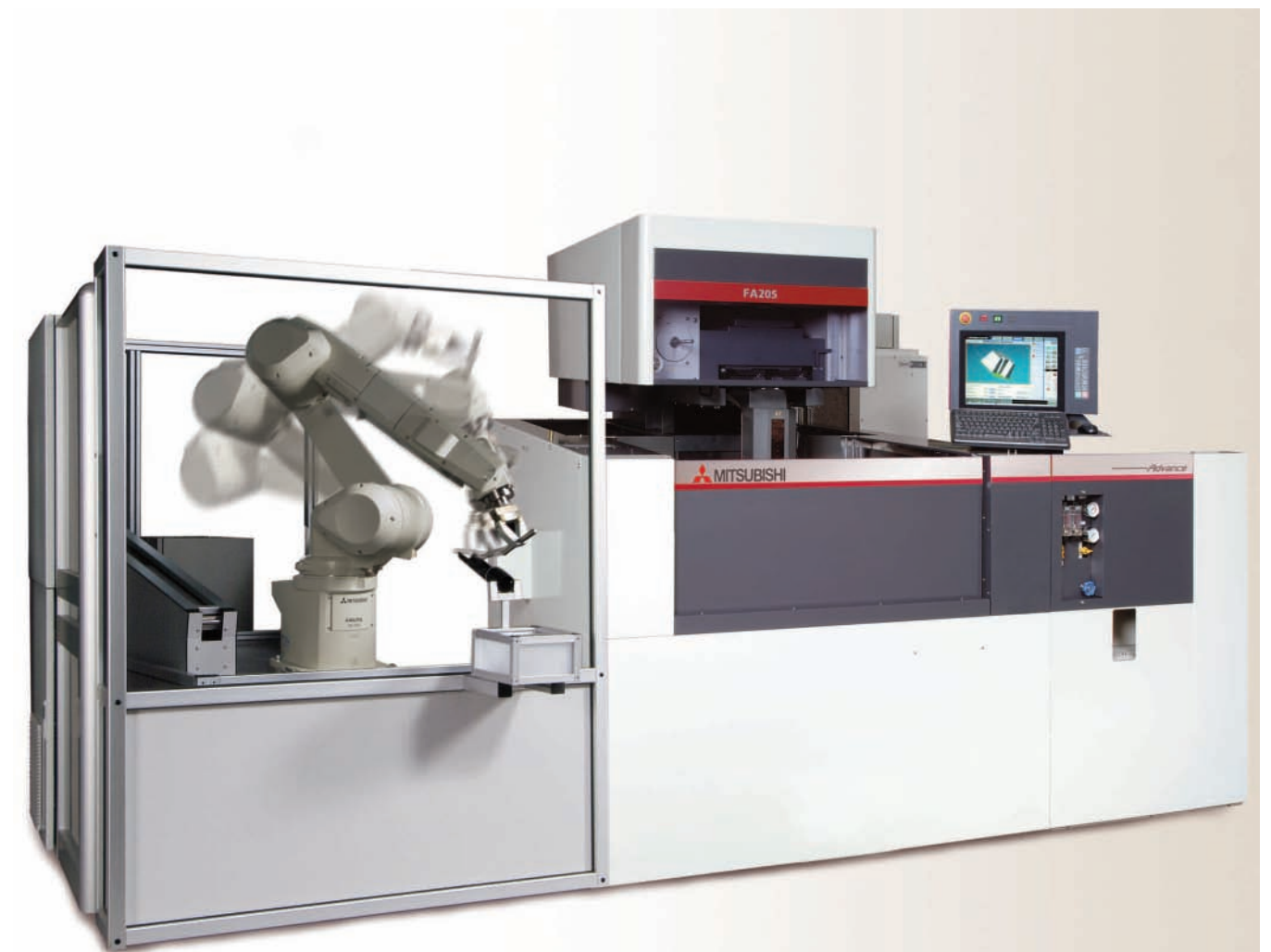
The figure shows the wire eroding system FA20-S Advance, automated with the MitsubishiRobot RV-12SL.
