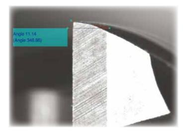
Cylindrical cutter with 4 cutting edges, diameter 6mm. Front view: checking back rake angles (1° and 2°), required to guarantee finish cutting without vibrations affecting the material being processed.
