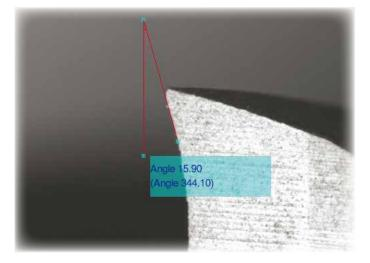
Cylindrical cutter with 3 cutting edges, diameter 10mm. Front view: front extent rake (rake angle) determines the performance of tool's working conditions.
