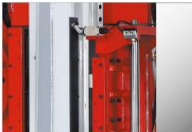
Heavy duty linear guides
