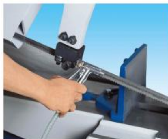
•清潔水槍 Cleaning Water Pipe
