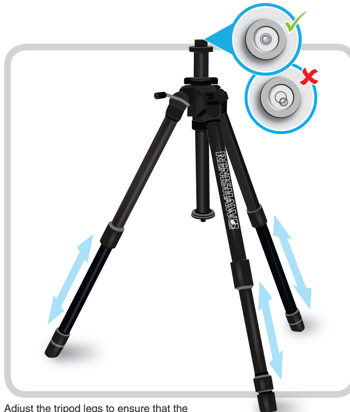
Adjust the tripod legs to ensure that the bubble is level
