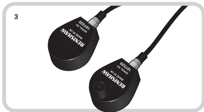
3 Position the sensors on the machine – the air sensor should be along the laser measurement path – the material sensors should be as close as possible to the machine drive. If difficult they can also be placed along the laser measurement path
