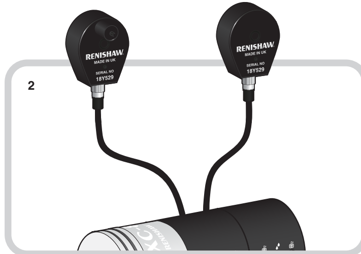
2 Connect the air and material sensors to the XC environmental compensator
