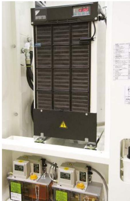
**Centralized Maintenance Cabinet** All critical maintenance items - lubrication reservoirs, oil chiller, air delivery - are easily accessible for inspection and routine service in a conveniently located cabinet.
