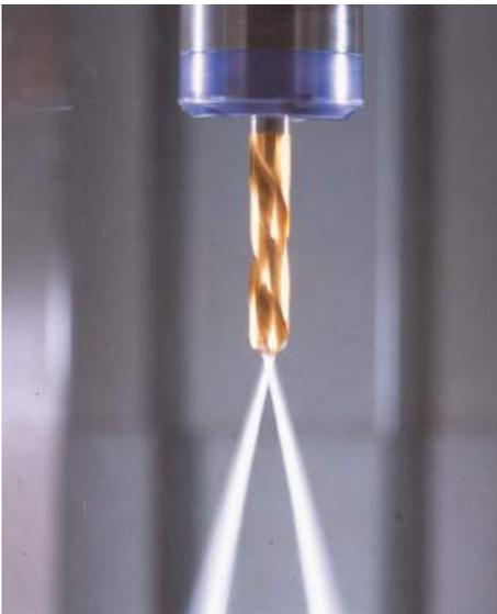
Coolant Through Spindle
