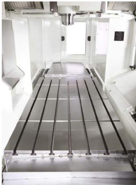
These large working areas in combination with heavy table load capacities up to 6,000kg (13,227Lbs) allows the Bridgecenter-G Series to achieve excellent performance on heavy duty cutting of molds to high accuracy cutting of precise parts.
