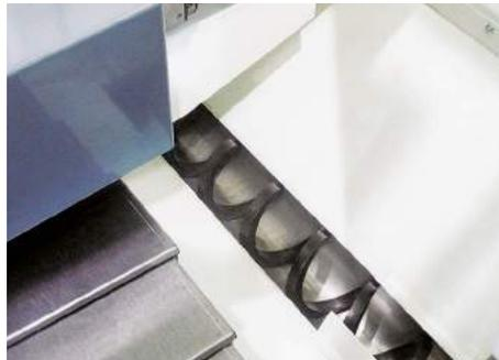
A chip-free machining environment boosts productivity and machining accuracy. A high-efficiency chip management system with overhead wash and base wash coolant and an auger style chip evacuation system is standard. A caterpillar style chip conveyor is an available option.
