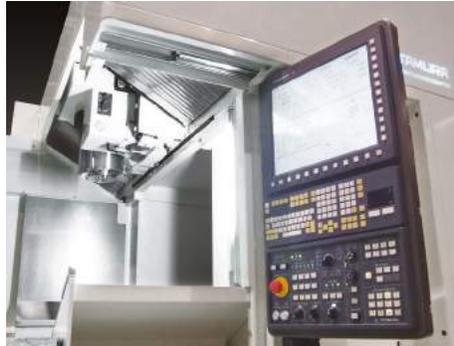
The Bridgecenter Series provide spacious working areas with ample table sizes up to 1,370mm (53.9") x 3,500mm (137.8") and Y-Axis travel of 1,615mm (63.6").
