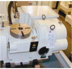
Field Retrofittable 4th and 5th Axis Rotary Tables
