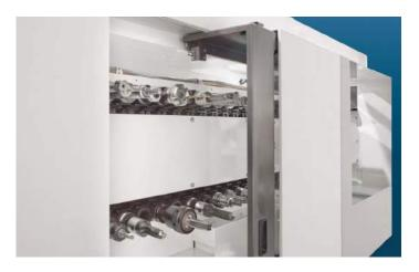
Efficient, ultra-high speed tool handling slashes idle time to maximize machining profit. Kitamura Mytrunnion 5-Axis machining centers employ a memory-random tool selection system for smooth idle-free tool changes. Generous 60T (100 opt.) ATC is conveniently located for optimum operator accessibility, offering flexibility in the parts you produce.
