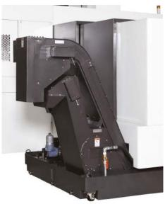
High Capacity, Double-Decker Chip Conveyor
