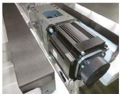
Premium grade servomotors with 16 million pulse encoders deliver astounding +/- 0.002mm (+/-0.000079") / full stroke positioning accuracies and powerful drive capability for tough cutting conditions.
