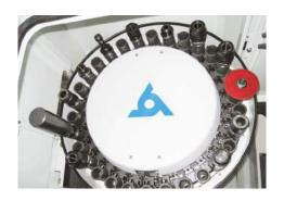
Efficient tool handling slashes idle time to maximize machining profit. The use of a memory-random tool selection system assures smooth idle-free tool changes. Its generous 30 tool ATC enhances machining capability.
