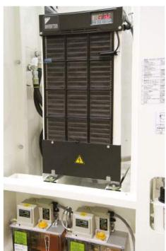
Centralized Maintenance Cabinet All critical maintenance items - lubrication reservoirs, oil chiller, air delivery - are easily accessible for inspection and routine service in a conveniently located cabinet.
