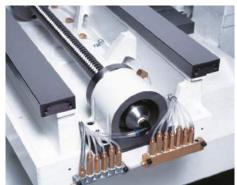
High-precision, pre-tensioned fine pitch ballscrews are precisely temperature regulated to eliminate accuracy robbing thermal growth.
