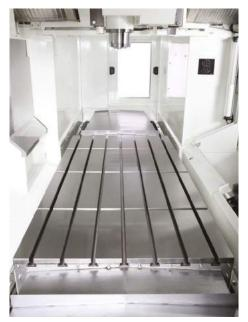
These large working areas in combination with heavy table load capacities up to 6,000kg (13,227Lbs) allows the Bridgecenter-G Series to achieve excellent performance on heavy duty cutting of molds to high accuracy cutting of precise parts.
