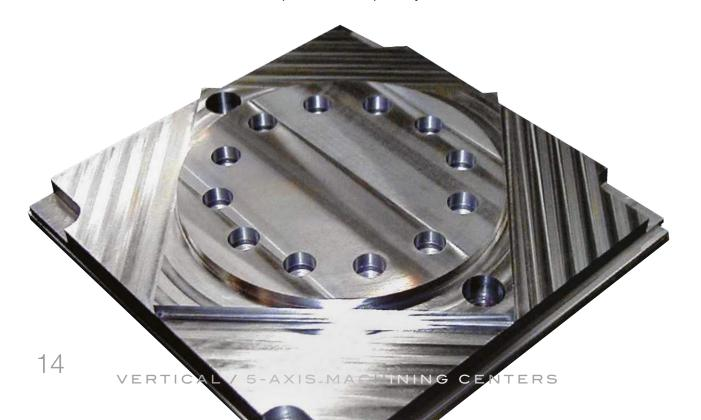
Designed to maximize load and unload of workpieces when the machine is in cycle, the safety and efficiency of workpiece handling, Kitamura's factory installed 2-station, 180 degree rotating pallet changer incorporates fully automatic operation with a quick and consistent 9.3 second pallet change time. With the integration of the pallet changer into a space saving work envelope, Mycenter Sparkchangers are ready for applications that require fast change over at a moment's notice.
