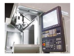
The Bridgecenter Series provide spacious working areas with ample table sizes up to 1,370mm (53.9") x 3,500mm (137.8") and Y-Axis travel of 1,615mm (63.6").
