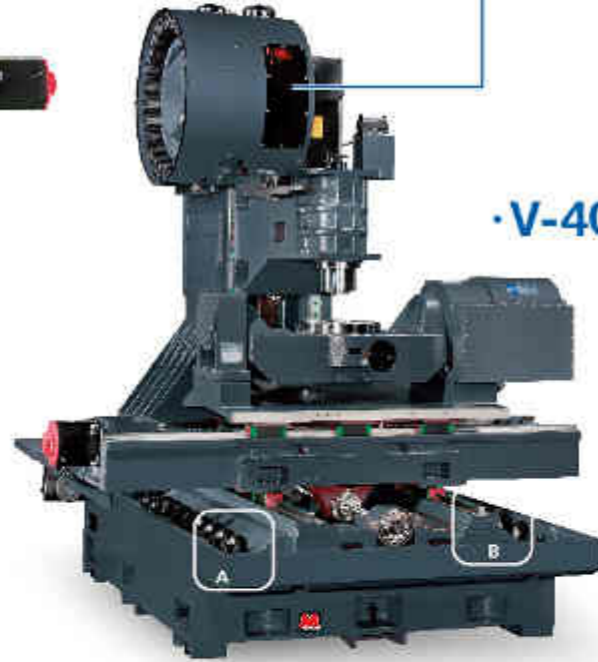
Lower the ATC magazine for shipment
