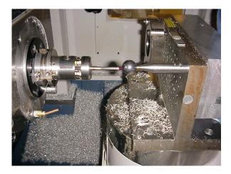
The probe's diminutive size allows small machine users to benefit from the high accuracy of strain gauge technology for the first time. The OMP400 is suitable for use on machines with short Z-axis travel and spindles as small as HSK32.
