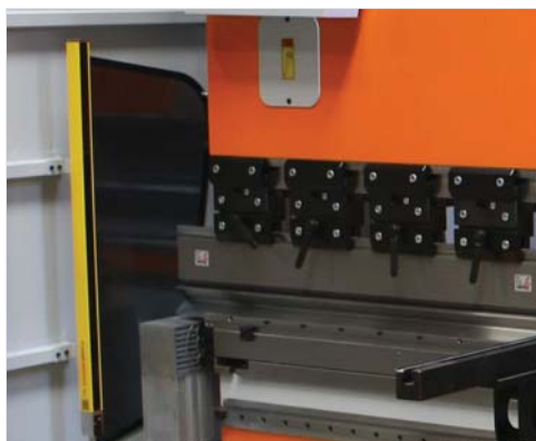
■ Body protection light curtain compliant with the CE standards ensuring safe operation (S)
