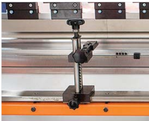
■ Specially designed folding backgauge fingers (S)
