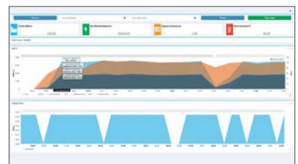
■ PRODUCTION AND ENERGY CONSUMPTION SCREEN During production, the machine's energy consumption allows the number of parts produced and hydraulic oil temperature changes to be monitored.
