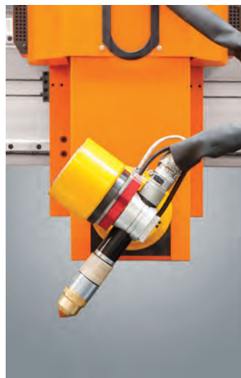
■ Can move totally +50 and 60° degrees at A axis.
