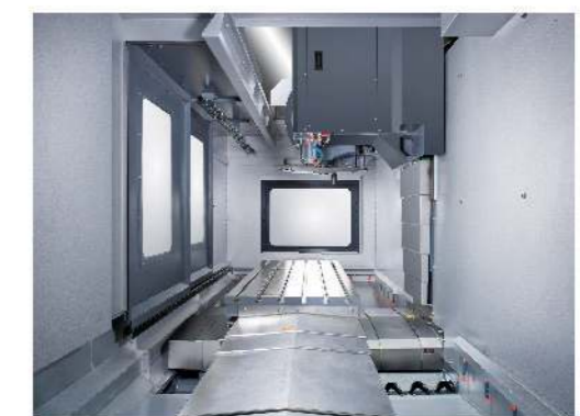
Surrounding coolant system
