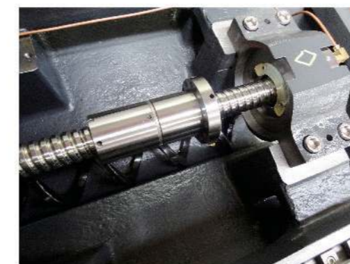
Dual nuts ball screw design in X and Y axis
