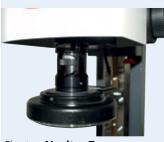
Six step **Navitar Zoom lens-Objektiv** with 0.7-4.5x magnification
