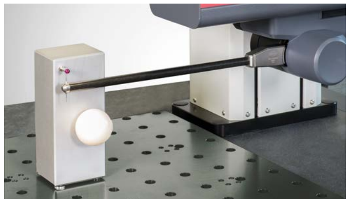
Greater reliability: user-guided calibration process with 2-sphere calibration standard
