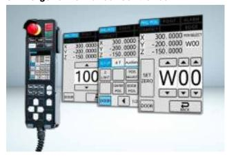
The ergonomically designed, intelligent manual control box unites all the relevant functions for control and set-up in a single unit. The integrated LCD display can be individually configured by the operator. Inclusive of buttons for driving all 8 possible CNC axes.
