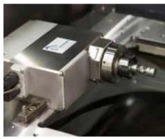
A servo-controlled B-axis fully integrated in the machine controls permits wire cutting on a rotating carried workpiece. Separation and multi-sided machining can be performed in a single clamping as well as simultaneously.
