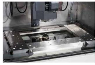
The three-sided work table is ergonomically built on the Z=0 level. This way workpieces can be perfectly positioned, even without clamping elements. High-grade stainless steel components and the stainless steel tank ensure dependability and maintenance-freedom.
