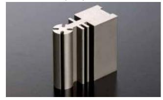
4 cuts of Ra 0.30 µm compared to a conventional machine.
