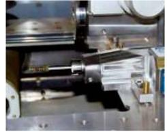
Rotating spindle fully integrated in the machine control with positioning for the most minute high-precision components, e.g. the manufacture of ejector pins with a diameter of ≥ 0.05 mm, the realisation of conical threads in medical technology, erosive grinding, turning and simultaneous machining.
