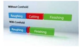
During roughing, the EDM system separates the part from the waste, but after cutting joins them together again with one or more dot welds. After this, the waste pieces can be removed from the workpiece and collected. The machining programme can then be resumed. On long-running jobs with multiple cut-outs, machine running time is therefore considerably reduced.
