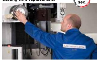
Simply replace the spool and feed the cutting wire over the feed rollers. Everything ready for work again in 92 seconds.
