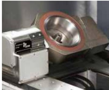
Machining cones to the highest standards of precision: the rotational/swivel axis integrated in the machine controls. Multi-axis machining to the centre of the workpiece and multi-sided machining in a single clamping, plus the realisation of high-precision conical polygons.
