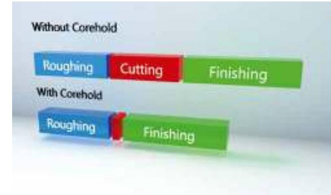
During roughing, the EDM system separates the part from the waste, but after cutting joins them together again with one or more dot welds. After this, the waste pieces can be removed from the workpiece and collected. The machining programme can then be resumed. On long-running jobs with multiple cut-outs, machine running time is therefore considerably reduced.
