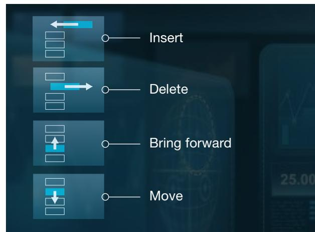
This is the easy way to add new jobs during machining or change the order of existing machining operations. The new job processing system with priority management makes it possible to amend a machining list without interrupting machining.
