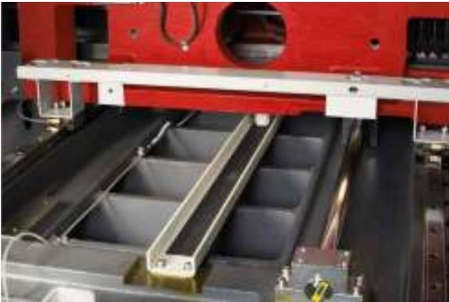
What was it about the main X and Y axes of conventional drive systems that bothered developers at Mitsubishi Electric? The need for lubrication, the friction and frictional heat, power consumption, backlash, the cogging moment and above all the possible wear. Only a non-contact drive overcomes these drawbacks from the outset and is thus an assurance of better results and enhanced dependability over decades.
