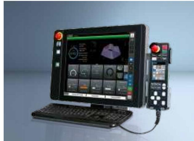
... simply shifts the future into the present. The user has almost half a metre of user interface to work with, assisted in this by the mouse and the usual computer keyboard. The monitoring of the machining process generates neatly displayed information at a glance and detailed analysis where desired.
