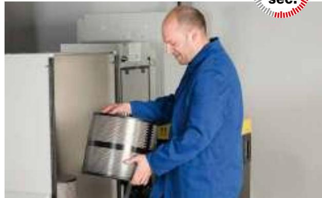
...without tools or wasted time. Two hands, 32 seconds – and the filter is replaced.
