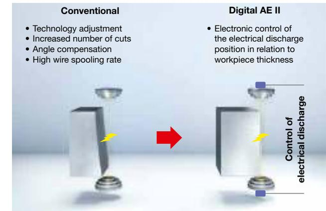
With precise control of the electrical discharge position, material is only removed where it needs to be. The patented functions of the Digital AE II improve rough and fine machining and fine finishing – in terms of both precision and machining time.
