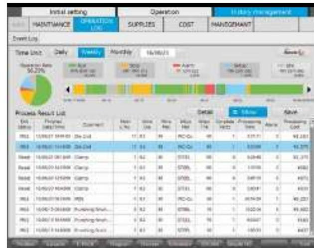
Machine states depicted over time make capacity utilisation easier to grasp and assist forward-looking production planning. This overview is supplemented by a list of completed machining jobs and the associated machine times and unit costs.
