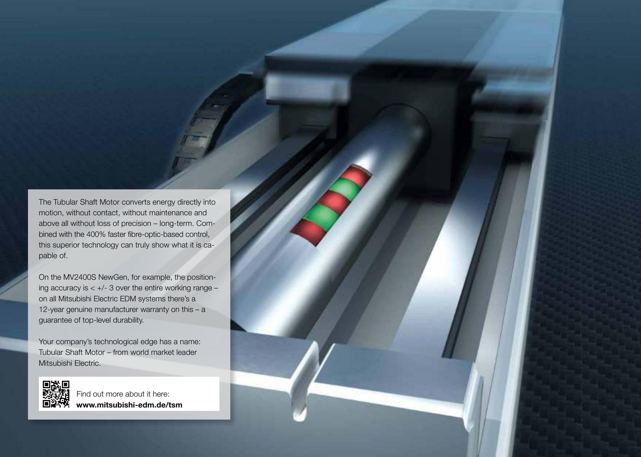
The Tubular Shaft Motor converts energy directly into motion, without contact, without maintenance and above all without loss of precision – long-term. Combined with the 400% faster fibre-optic-based control, this superior technology can truly show what it is capable of.
