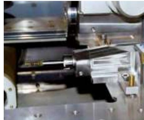
Rotating spindle fully integrated in the machine control with positioning for the most minute high-precision components, e.g. the manufacture of ejector pins with a diameter of  $\geq 0.05$  mm, the realisation of conical threads in medical technology, erosive grinding, turning and simultaneous machining.
