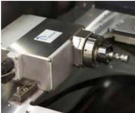
A servo-controlled B-axis fully integrated in the machine controls permits wire cutting on a rotating carried workpiece. Separation and multi-sided machining can be performed in a single clamping as well as simultaneously.
