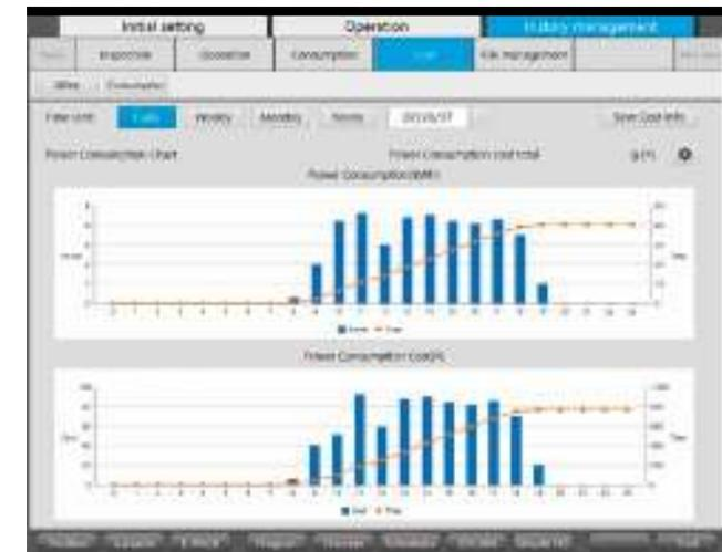
Given knowledge of unit costs and their inclusion in the machine's own analysis, records of consumption data such as energy consumption\*, wire consumption and component wear help with cost analysis and the costing of pending machining jobs.
