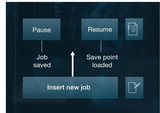
A machining process is easy to pause even in mid-flow when urgent jobs have to be processed. The control stores the current state of machining. When the inserted job has been completed, machining can be immediately resumed at the point of interruption. Pushbutton flexibility without programming effort.
