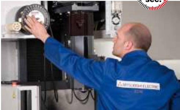
Simply replace the spool and feed the cutting wire over the feed rollers. Everything ready for work again in 92 seconds.
