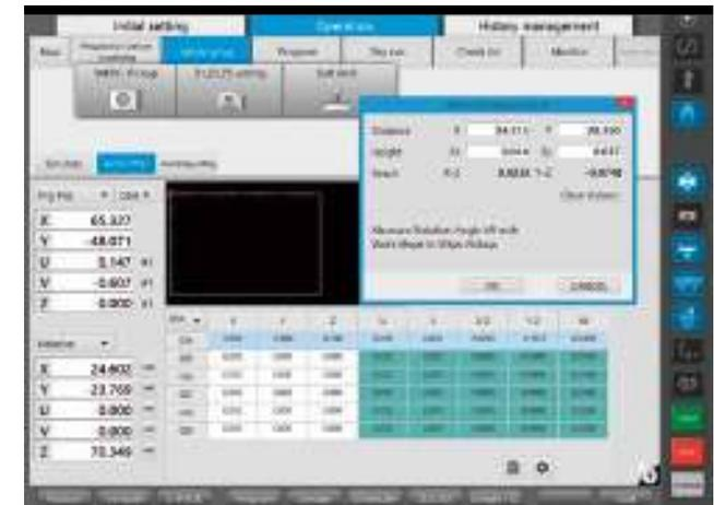
Both are possible. As a user, you decide whether you do set-up classically by hand or the machine automatically defines the position of your workpiece. Using the cutting wire or pick-up coil – the machine takes care of it for you. It only takes the press of a button.
