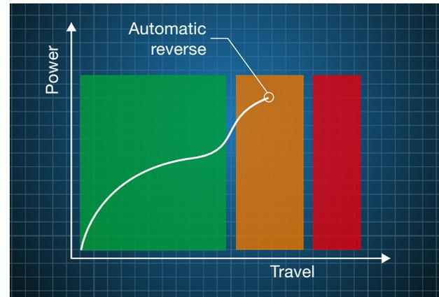
The wire-cut EDM systems from Mitsubishi Electric constantly check current axial forces and thus fully automatically detect potential accidents before they happen. If there is an obstacle in the travel path, this is electronically detected on the basis of the drive's load change during the approach and the control automatically reverses. Better safe than sorry!
