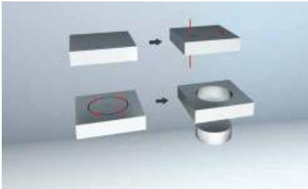
During roughing, a bridge is controllably created to hold the waste material – the waste material cannot fall. In this way many features can be rough-machined and, after removal of the waste material, recut – fully automatically and unmanned, overnight and at week-ends. Lower costs, higher profits.
