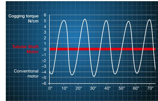
You're surely familiar with the cogging torque manifested by a conventional electric motor. It is precisely this cogging torque that is undesirable, as are variations in torque. The Tubular Shaft Motor – the optimal drive for precision applications like electrical discharge machining.
