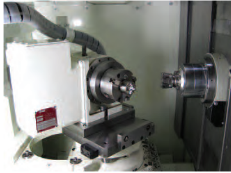
Field installed 5th axis capable on BOTH pallets.
