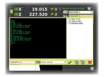
The datas are elaborated and post-processed by the software. There are more than 50 post-processor format for the most common numerical controls available on machine tool market.
