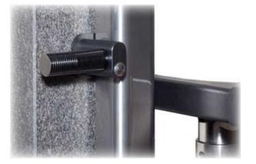
Manual axes movement. Axis unclamping by means of a single pneumatic control system.
