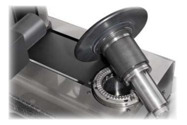
Interchangeable revolving spindle with mechanical rotation brake. Two preloaded ball cages allow a concentricity accuracy within 2 µm.
