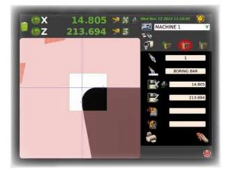
New electronic control: a powerful fanless PC with Linux operating system for the integrated management of the functions of measurement / inspection tools, machine origins and toolsets. Ease of use thanks to the integrated touch screen.
