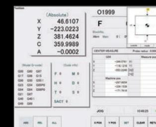
**Work Set Assistance.** Set-up work offsets with just a few keystrokes. Four types of measurements are possible. Edge side measure, center measure, 3 point diameter center measure and corner measure if angular.
