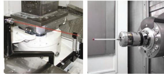
Spindle and Tool Probes
