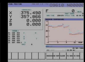
**Intelligent Advanced Control System.** Controls the effects of heat displacement in order to ensure continuous accuracy in machining. Minimizes head displacement to less than  $\pm 5$  microns. 6 sensors positioned on the machine measure and monitor temperature of machine and compensation guarantees positioning accuracy of  $\pm 0.002\text{mm}$  ( $\pm 0.000079$ ") / Full stroke. Kitamura patented system since 1998.
