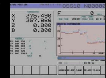
**Intelligent Advanced Control System.** Controls the effects of heat displacement in order to ensure continuous accuracy in machining. Minimizes head displacement to less than +/-5 microns. 6 sensors positioned on the machine measure and monitor temperature of machine and compensation guarantees positioning accuracy of +/-0.002mm (+/-0.000079") / Full stroke. Kitamura patented system since 1998.
