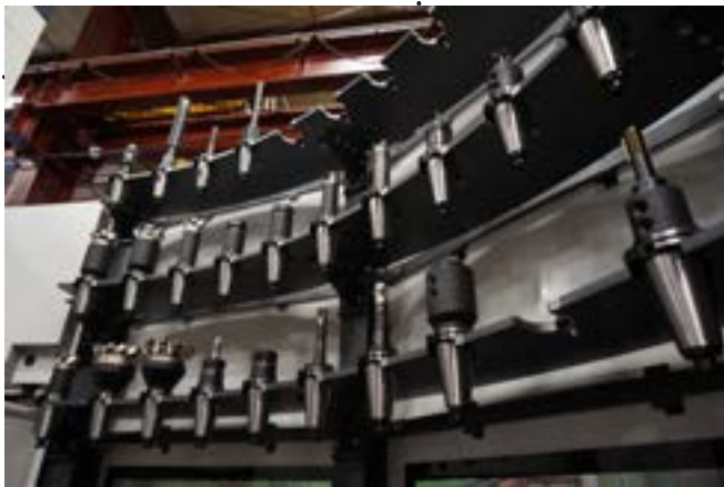
Robotic Tool Changer - Max. Capacity 210 tools
