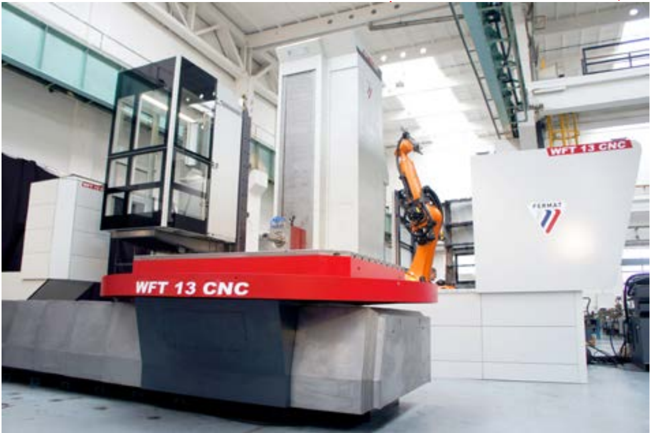
WFT 13 CNC with KUKA Robot and new Pickup Station for Milling Heads
