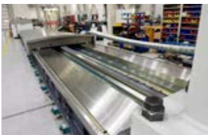
X-Axis Hydrostatic guideways
