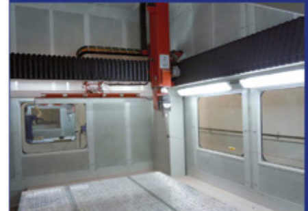
Aluminium vacuum table with T slots Piano aspirante in alluminio con cave a T
