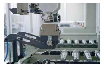
Integrated heavy-duty gantry loader and workpiece conveyor
