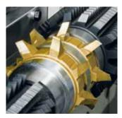
Chamfering/deburring with chamfer hobs
