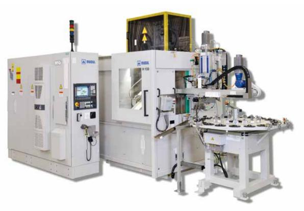
H 80 – H 200 Universal gantry loader for direct feed from various work piece storage systems and automation devices. Easy integration into manufacturing cells and systems.
