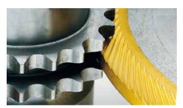
Deburring of chain sprocket gears
