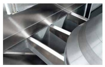
Stainless steel workarea enclosure for dry hobbing
