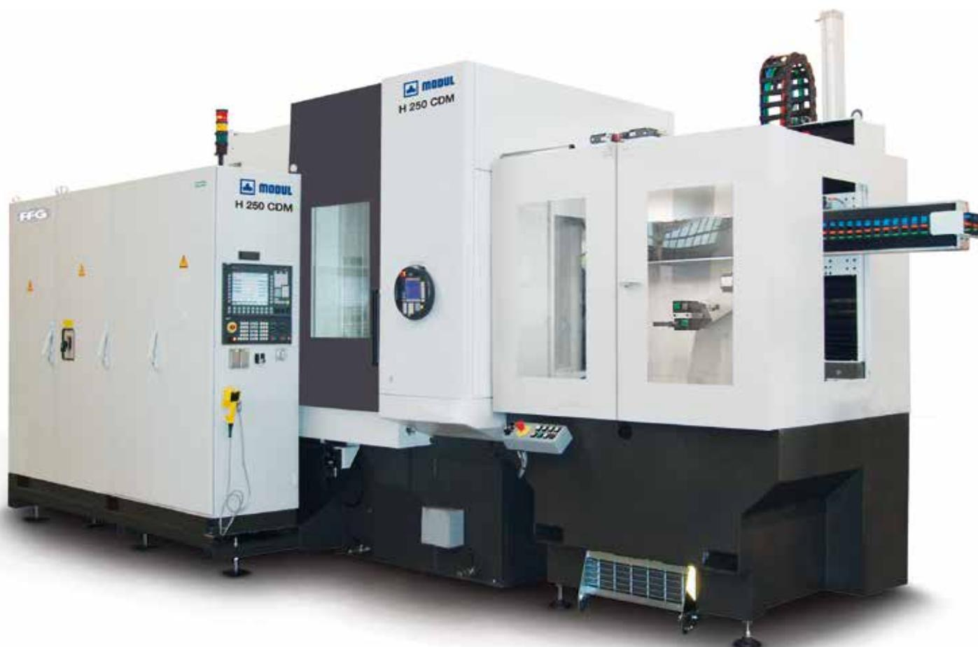
Combined hobbing and chamfering/deburring machine
