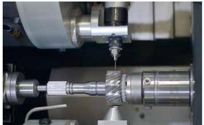
Integrated unit for the drilling of lubrication channels in one setup
