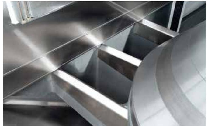
Stainless steel workarea enclosure for dry hobbing
