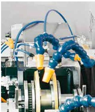
Horizontal workpiece axis for optimum residue fall
