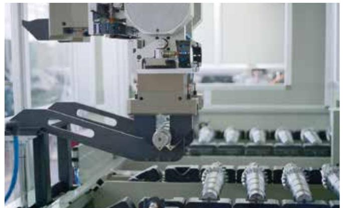
Integrated heavy-duty gantry loader and workpiece conveyor
