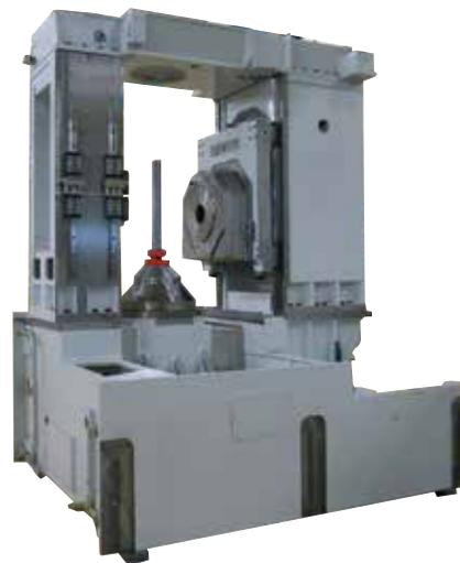
The closed frame structure ensures maximum rigidity
