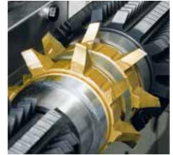
Chamfering/deburring with chamfer hobs
