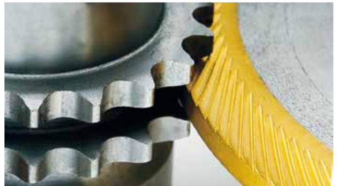
Deburring of chain sprocket gears
