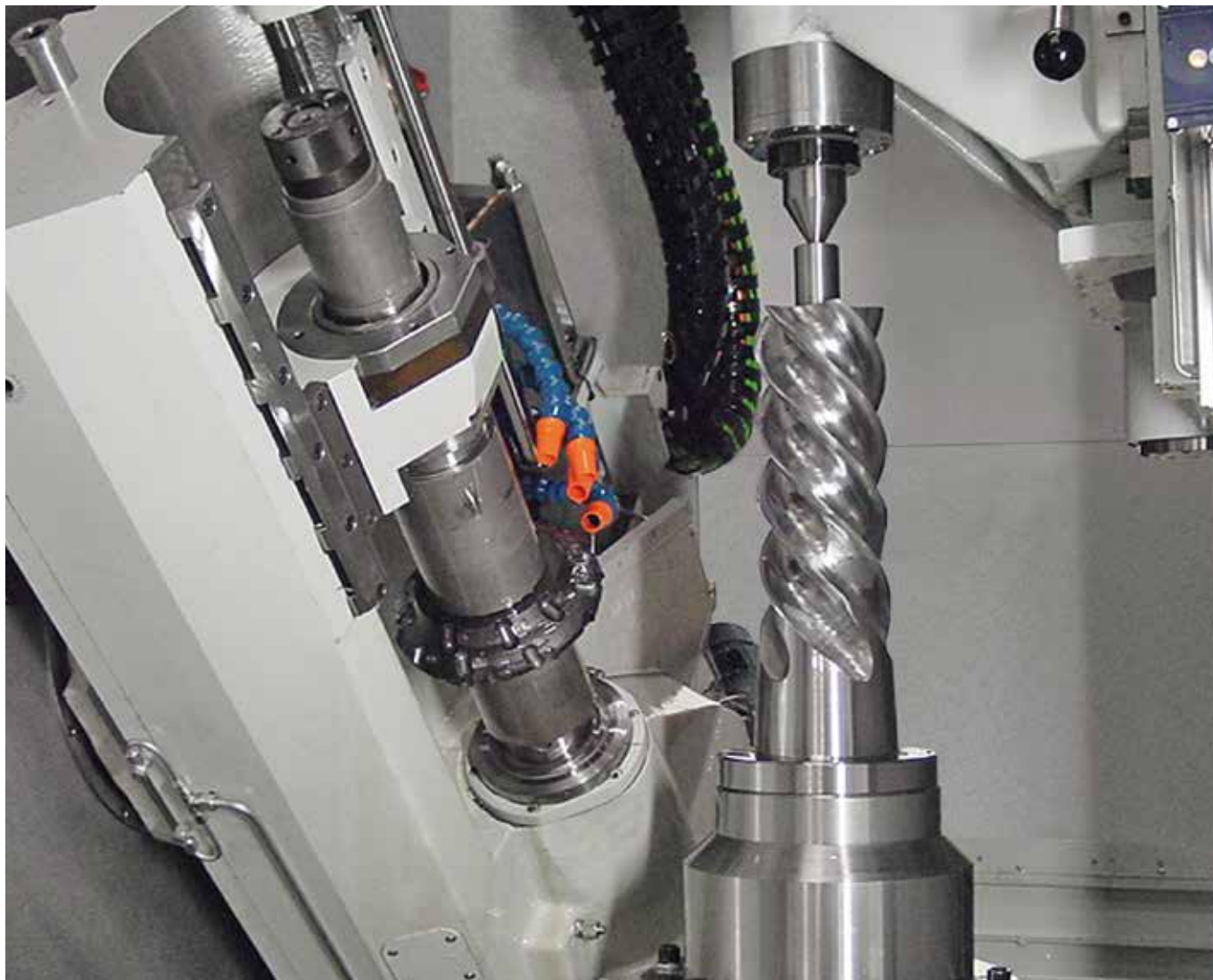
The H 600 equipped with PowerCutting options is especially suited for the milling or hobbing of large rotors
