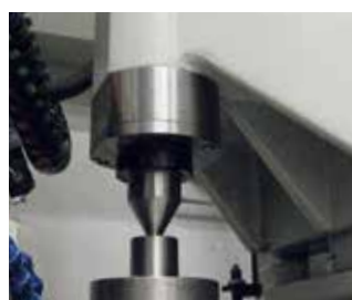
Automated tailstock with cam-free adjustment
