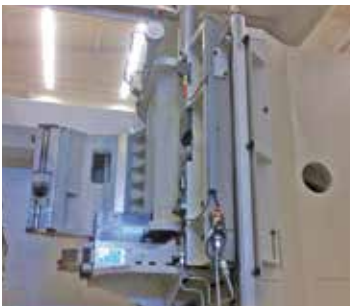
Swing-away tailstock arm and steady rest
