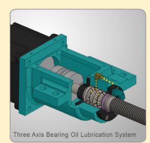
All three axis, and the bearing all have the automatic lubrication system installed. The life of the parts will be prolonged with this system. Not only get better rigidity, also reduce the thermal elongation.
