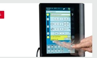
Simple Drag & Drop tasks and saved ISO tolerance tables make it very easy to create measuring programs.
