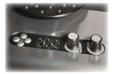
Stepper motors servo control the axes movements and provide two operation modes: rapid (2.5 m/min) and fine micrometric mode (positioning accuracy 0.8 µm).
