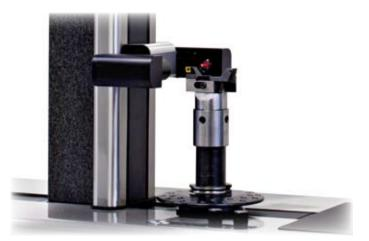
*Camera system for measuring and inspection procedures. C-MOS sensor, punctiform and toroidal red light double illuminator. Telecentric optic system with low F/Number.*
