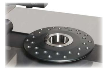
Spindle body with double ball retainer. Patented interchangeable spindle (run-out error < 2 µm). Universal shank locking system. Rotation brake. Angular index.
